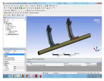
Figure 6: CAD model with boundary conditions.
