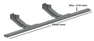
Figure 5: CAD model of an RUPD
